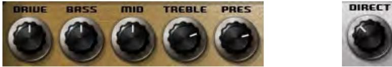
**DRIVE** controls the drive level range of +12dB to -12dBfs, with a default of 0dB.
