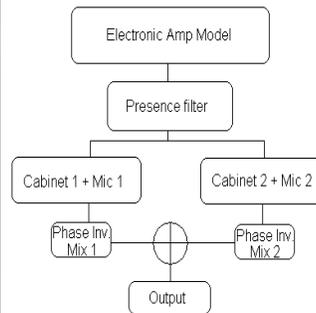
The Mono DualCab amp is similar to the Mono amp in that it inputs and outputs a Mono signal. The DualCab configuration lets you play the Amp's sound through two separate cabinets. This allows for combinations such as loading the same cabinet with different microphones or using two different cabinets with the same mic.
