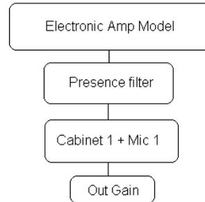
The Mono Amp is the least CPU-intensive of the Amp components. It inputs and outputs a Mono signal, running the output through a single Amp module and then into a single cabinet/microphone filter.
