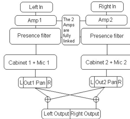
The Mono-to-Stereo and Stereo Amps share the same controls and graphic user interface, but their input and processing specifications are different.
