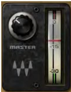
**MASTER VOLUME** controls overall output gain. Output meter includes red light clip indicator.
